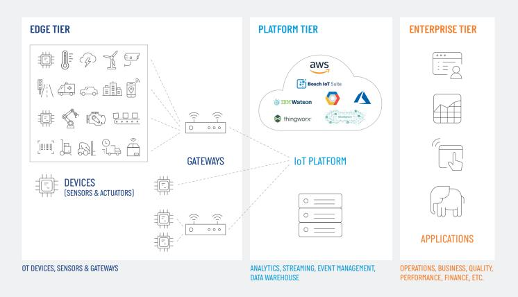
The first area, Edge Tier, which includes the OT or shop-floor IT, groups together all physical devices: from the sensor and actuator level to the control level and edge computing. It is also called the aggregation or orchestration level.
